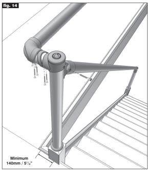
Simply mitre the handrails using the template supplied (found at the back of this booklet), slide them into the elbow from either side and check that the handrails pass the screw holes. Then pre drill and secure the handrails using the four screws supplied and glue from underneath (fig. 13).
